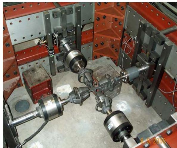
Figure 2: Biaxial test bench for cruciform specimens loaded in tension/tension.
