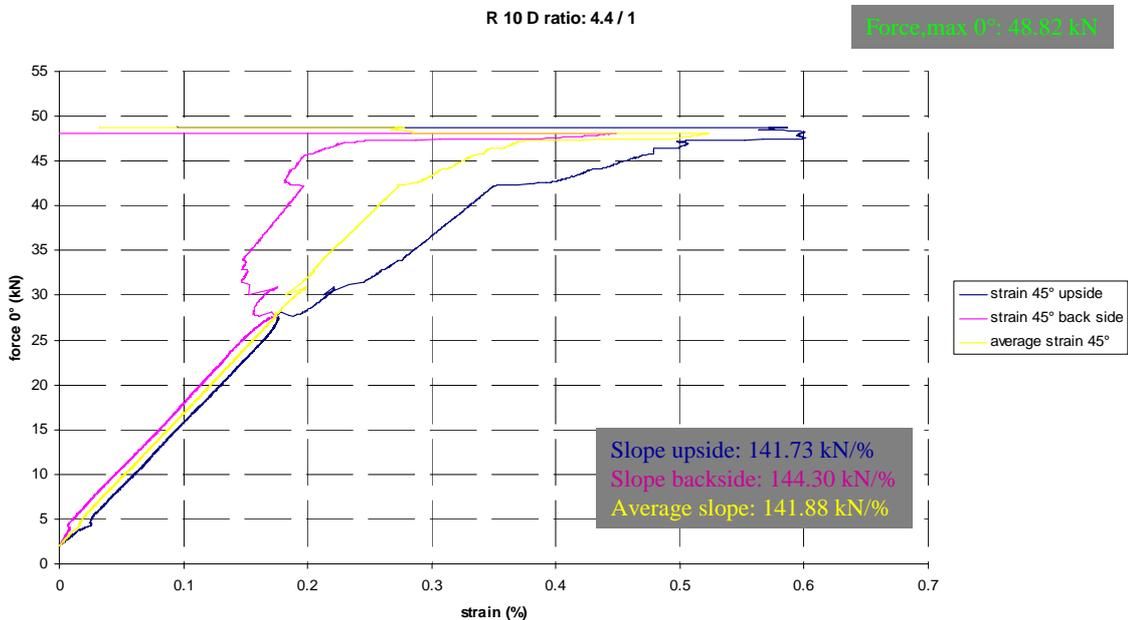
Graph 3c: Load in 0° direction vs. strain in 45° direction. R=10mm, Loading ratio=4.4/1.
