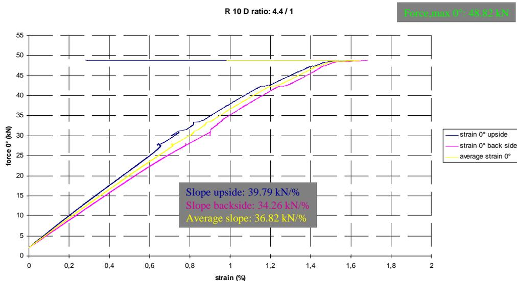
Graph 3a: Load in 0° direction vs. strain in 0° direction. R=10mm, Loading ratio=4.4/1.
