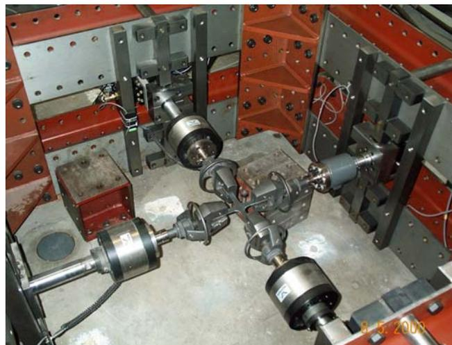
Figure 2: Biaxial test bench for cruciform specimens.
