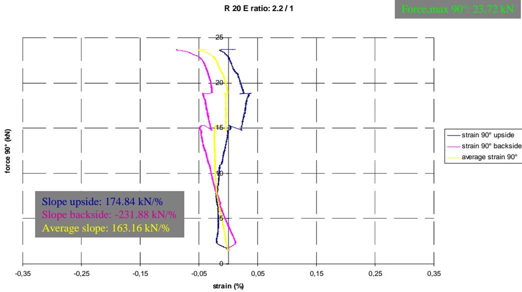
Graph 2b: Load in 90° direction vs. strain in 90° direction. R=20mm, Loading ratio=2.2/1.
