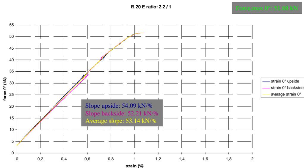
Graph 2a: Load in 0° direction vs. strain in 0° direction. R=20mm, Loading ratio=2.2/1.
