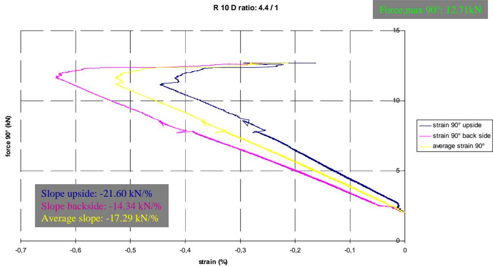
Graph 3b: Load in 90° direction vs. strain in 90° direction. R=10mm, Loading ratio=4.4/1.
