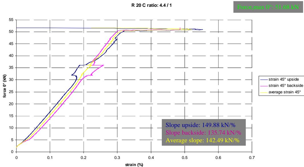
Graph 4c: Load in 0° direction vs. strain in 45° direction. R=20mm, Loading ratio=4.4/1.
