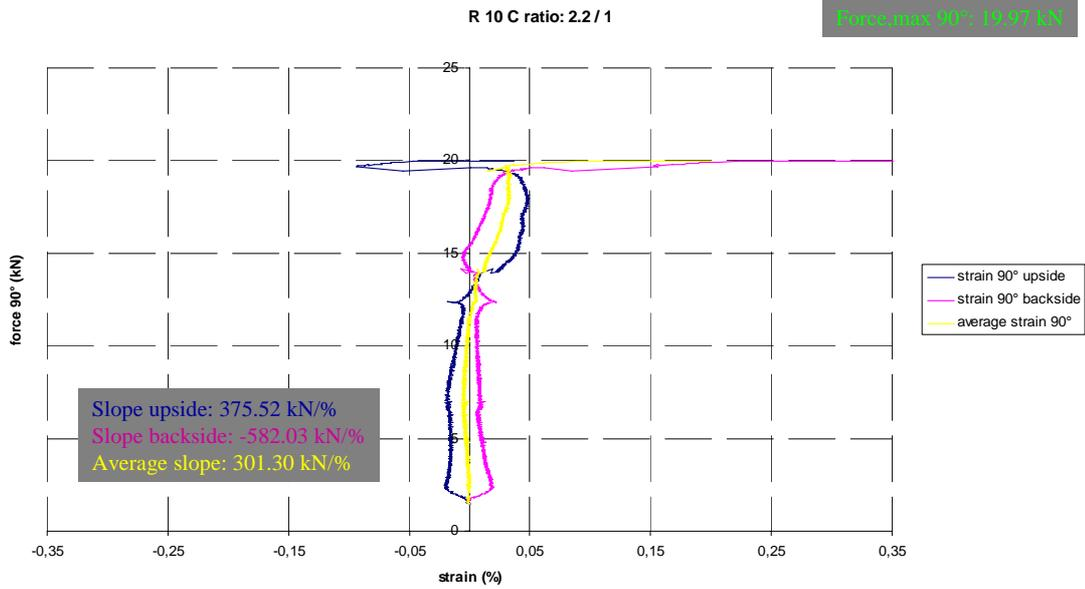
Graph 1b: Load in 90° direction vs. strain in 90° direction. R=10mm, Loading ratio=2.2/1.
