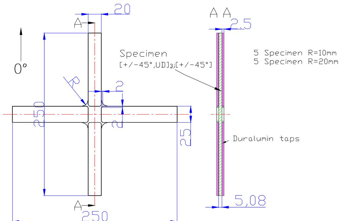
Figure 1: Geometry of cruciform specimens.
