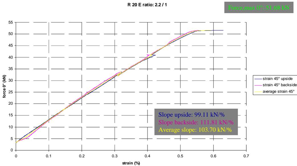
Graph 2c: Load in 0° direction vs. strain in 45° direction. R=20mm, Loading ratio=2.2/1.
