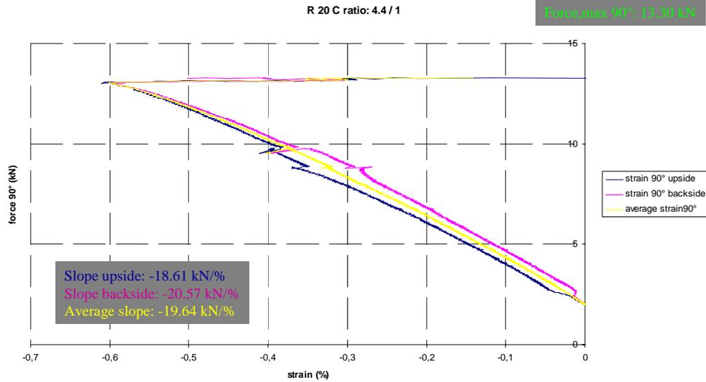
Graph 4b: Load in 90° direction vs. strain in 90° direction. R=20mm, Loading ratio=4.4/1.
