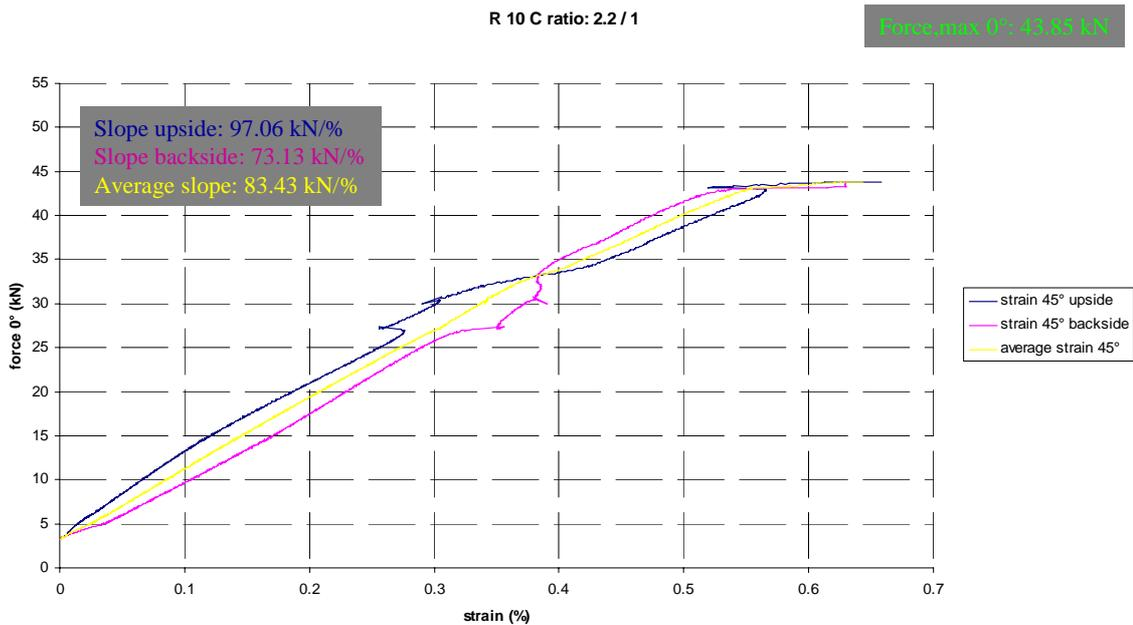
Graph 1c: Load in 0° direction vs. strain in 45° direction. R=10mm, Loading ratio=2.2/1.
