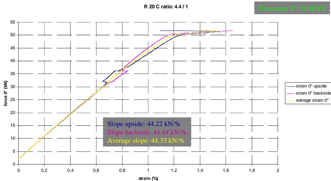
Graph 4a: Load in 0° direction vs. strain in 0° direction. R=20mm, Loading ratio=4.4/1.
