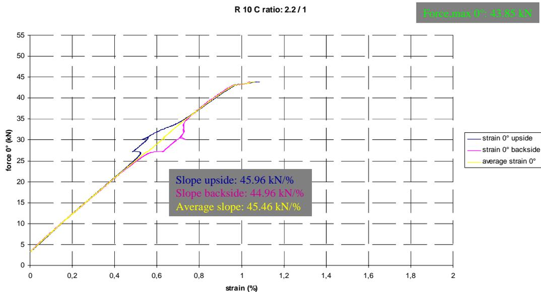
Graph 1a: Load in 0° direction vs. strain in 0° direction. R=10mm, Loading ratio=2.2/1.
