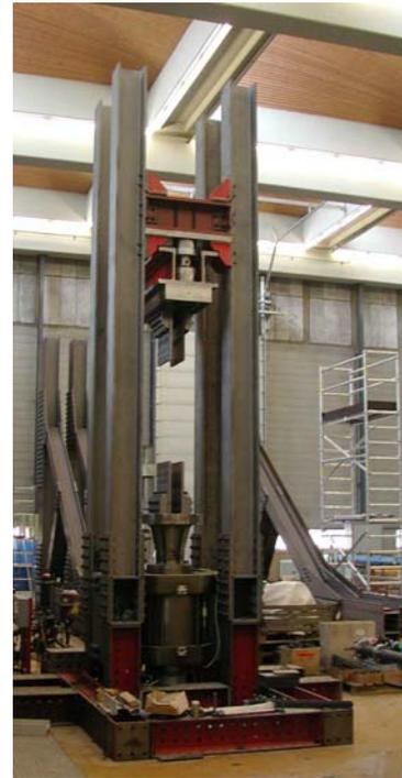
Figure 5 2500 kN test bench
