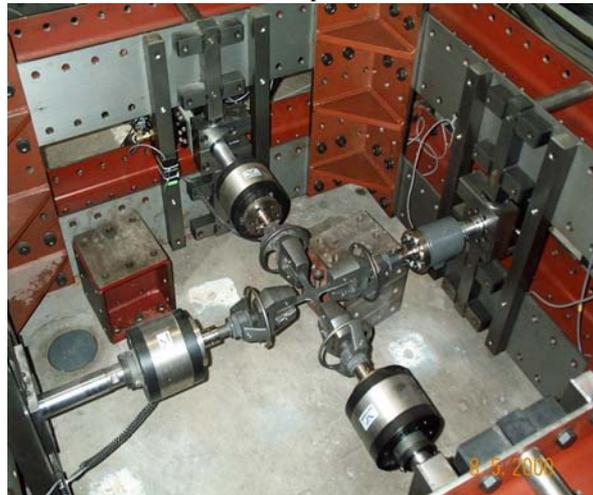
Figure 3 Bi-axial test set-up for tension-tension tests (VUB)
