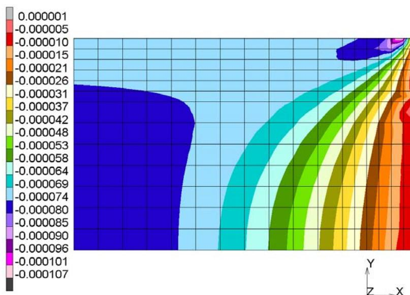
**Figure 12 Transverse strains for the MD specimen (OB\_TG4\_R004)**
