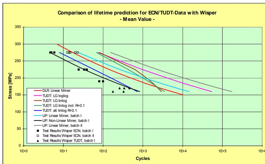
**Figure 8 Results of different lifetime prediction models of TUdT, UP and DLR**
