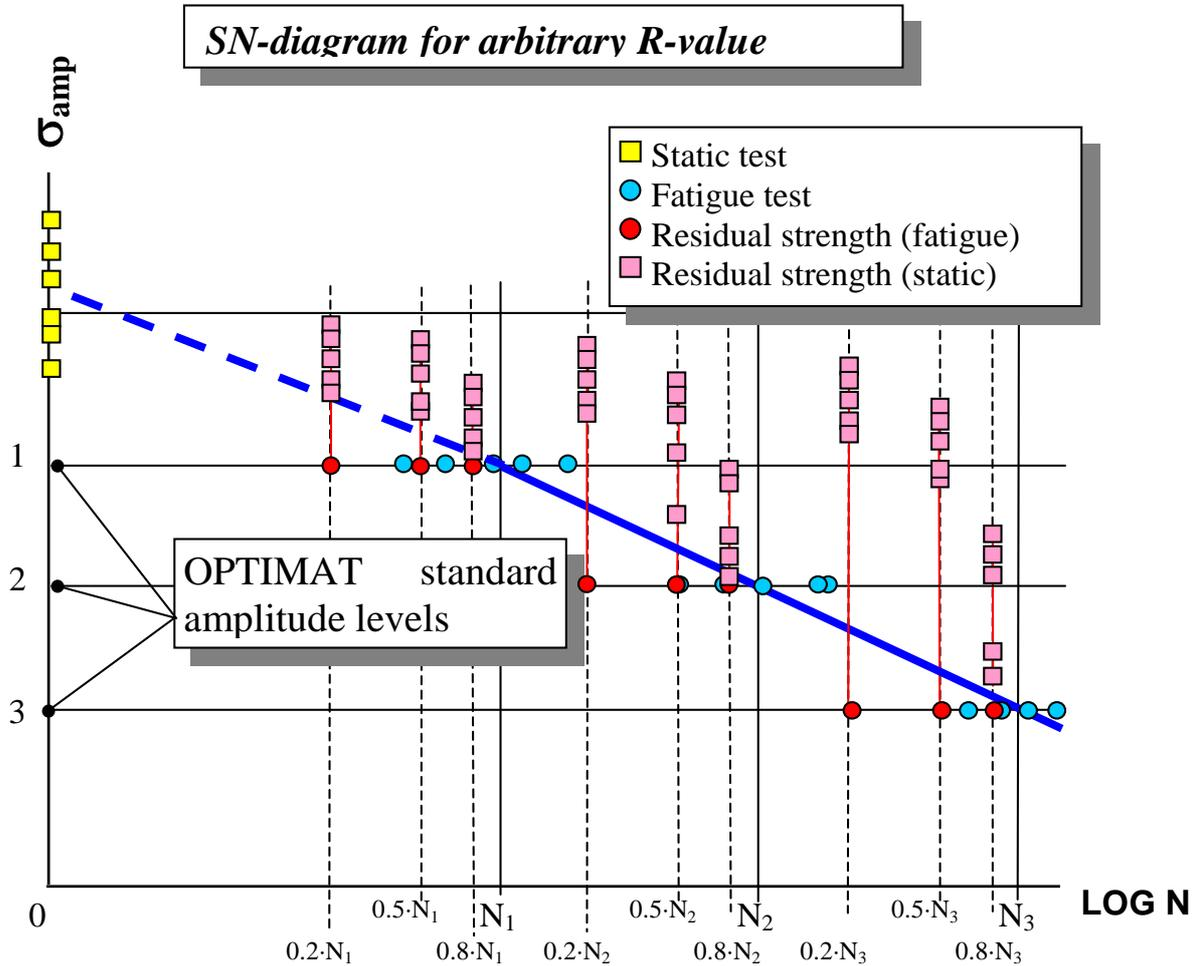
**Figure 18 Static, fatigue and residual strength tests**
