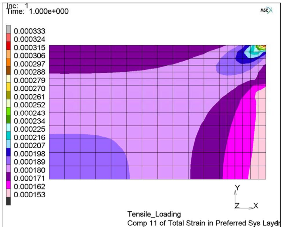
Figure 4 FE results of the MD test specimen
