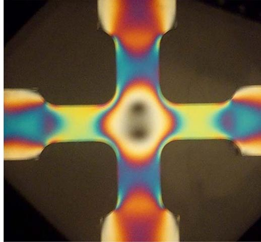
**Figure 9 ISOCHROMATICS in a transparent cruciform loaded biaxially.  $F_x = F_y = 300 \text{ N}$**
