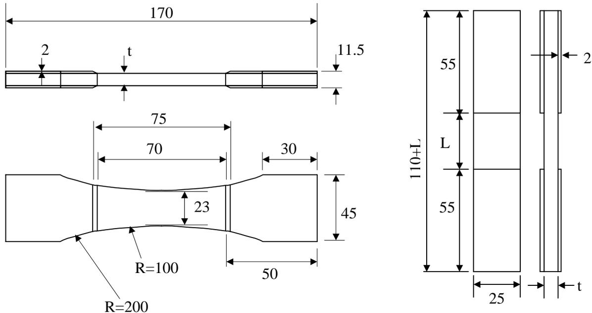
**Figure 1 Dimensions of specimens D01 (dog bone shaped, left) and R01**
