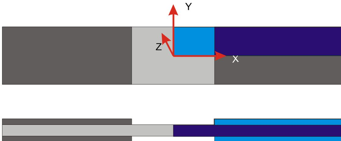
**Figure 2 FE model of the test specimen**
