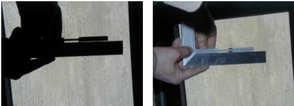
Fig. 3 Check of coupon's surface against a flat surface
