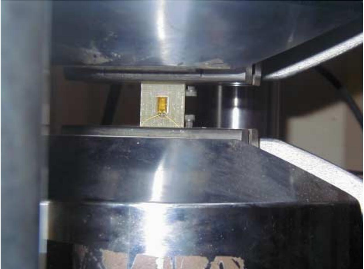
**Fig. 2 Setup of the coupon tests**
