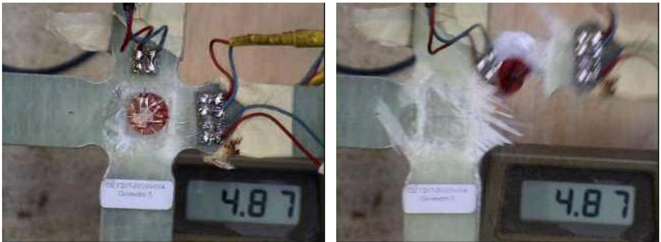
Fig.4 Cruciform specimen GEV 207 S0100-004 (geometry 5) at failure
