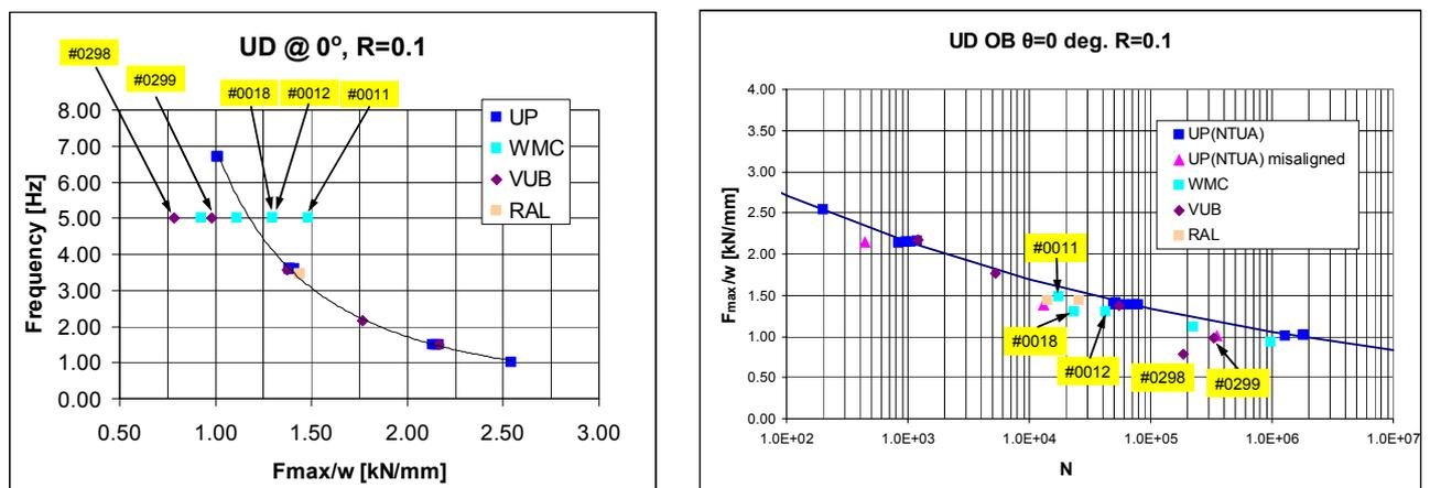
Fig.2 Sensitivity investigation of CA test results on frequency, coupon clamping & alignment, etc.
