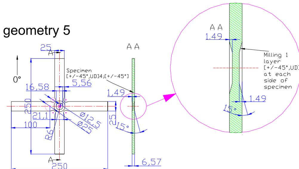
Fig.3 Preferred cruciform specimen geometry
