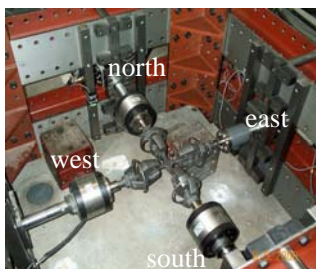
Fig. 1. Bi-axial test bench for flat cruciform specimens.
