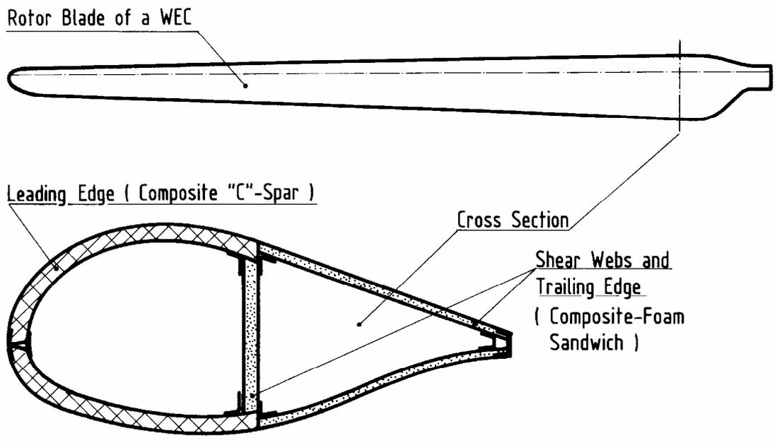
Figure 3: Structural details of a typical rotor blade
