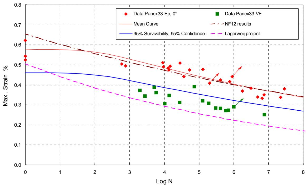
Figure 17: S-N curves of CFRP at R = -1 [24]
