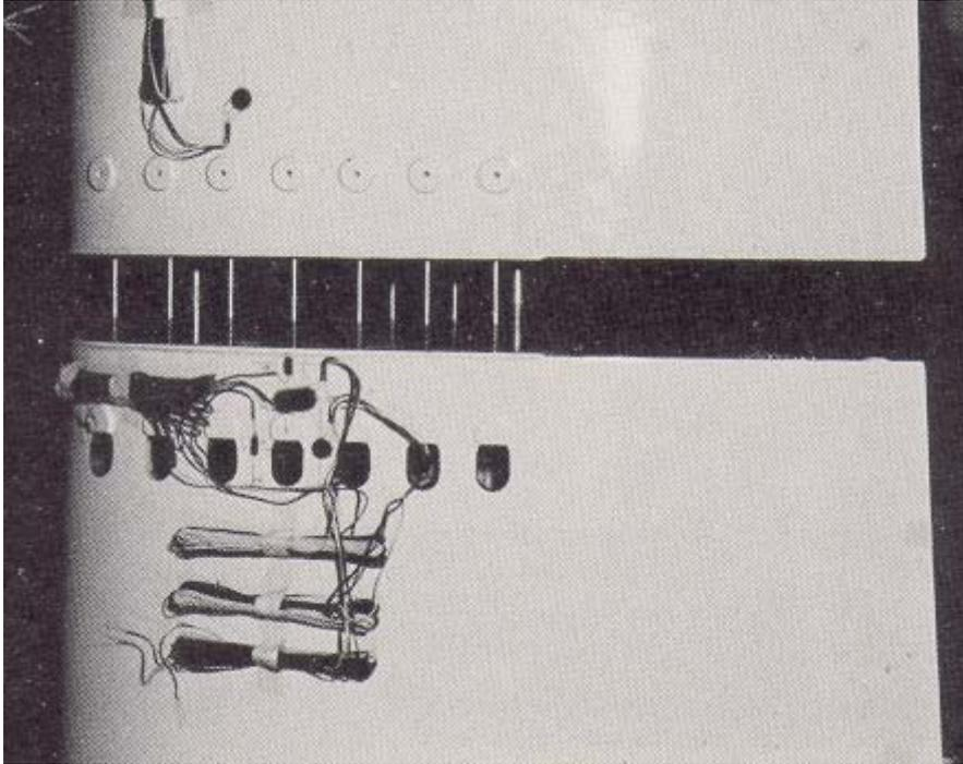
Figure 18: Picture of a T-bolt connection at the DEBRA 25 rotor blade [25]
