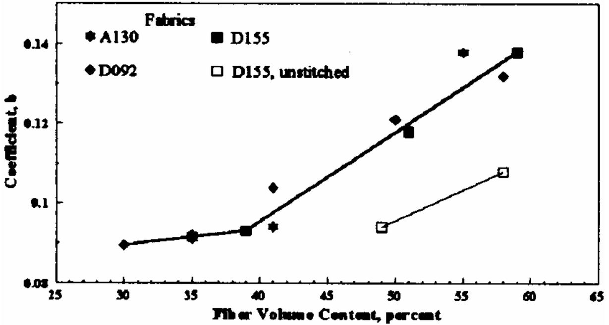
Figure 8: Influence of fibre content and fabric architecture on the slope of S-N curves [13]
