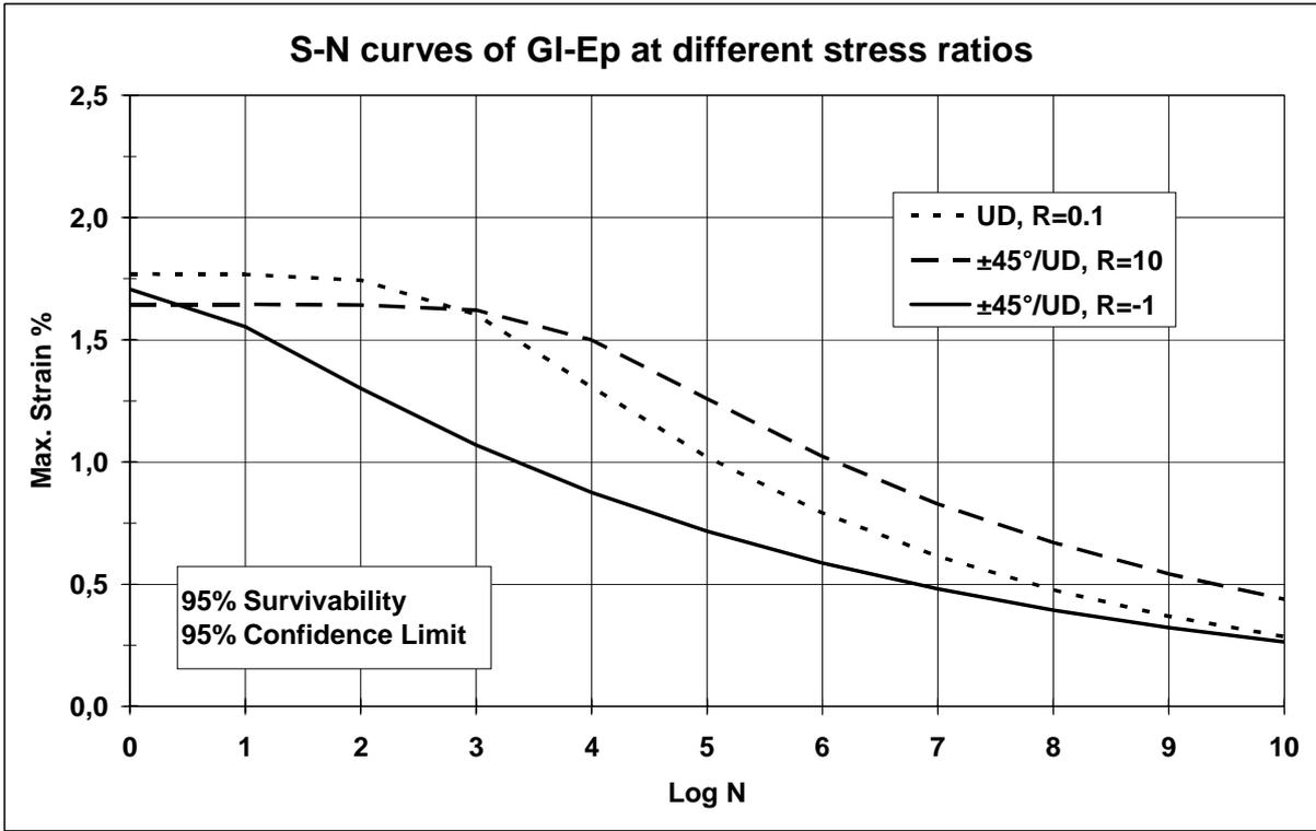
Figure 7: Example of S-N curves for GI-Ep at different stress ratios [8]
