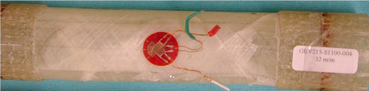
Figure 12: Delamination failure of overlap due to steep drop
