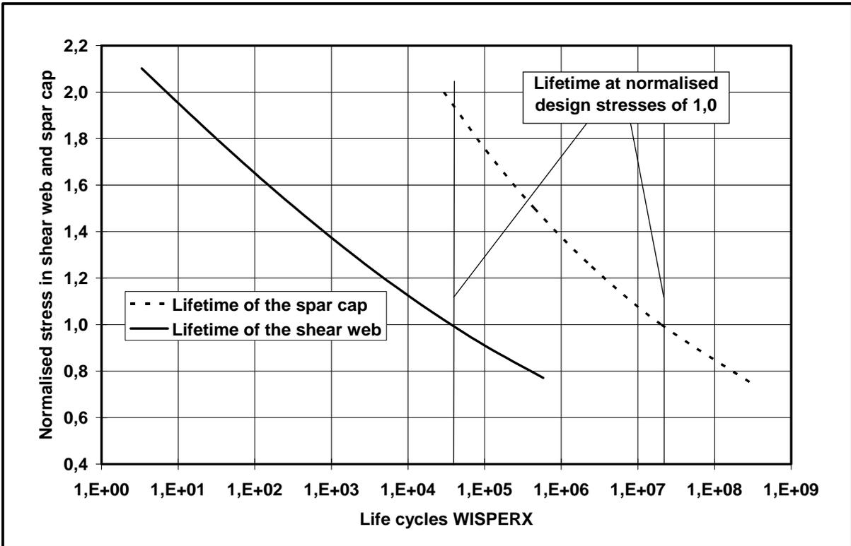
Figure 15: Lifetime comparison of a shear web and a cap of a GFRP-spar beam [15]
