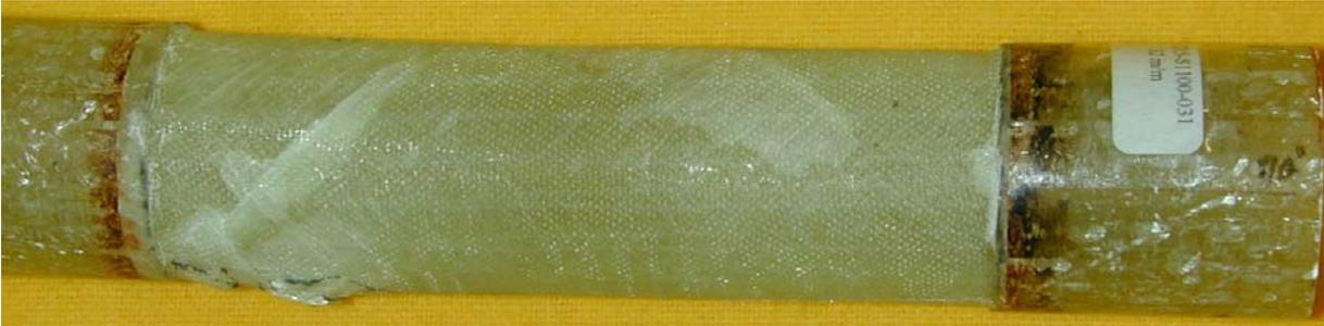
Figure 13: Improvement of failure mode with tapered overlap
