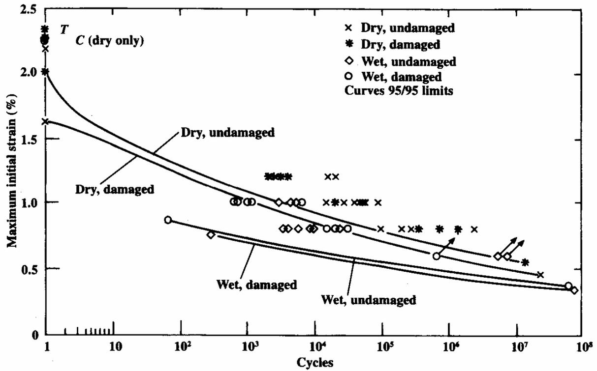
Figure 16: Environmental effects on the S-N curves of GI-Ep at R=-1 [23]
