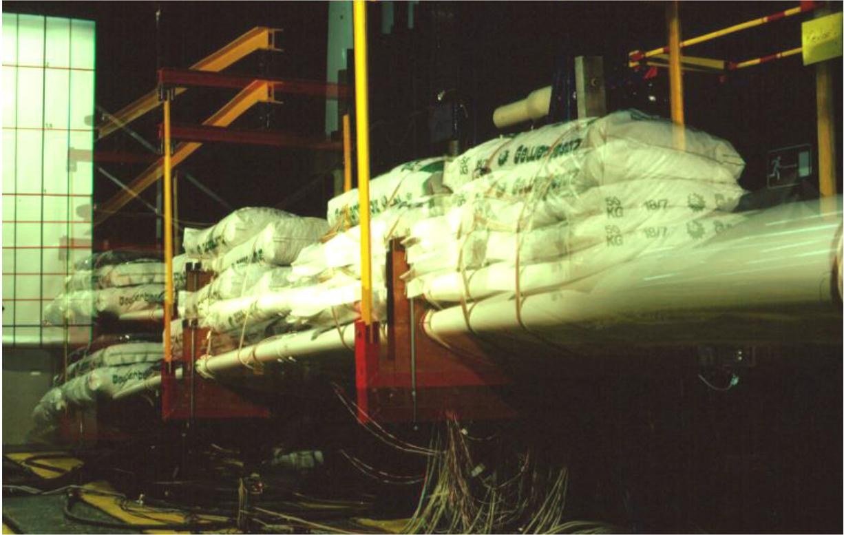
Figure 5: DEBRA 25 blade in test bed for service life investigation
