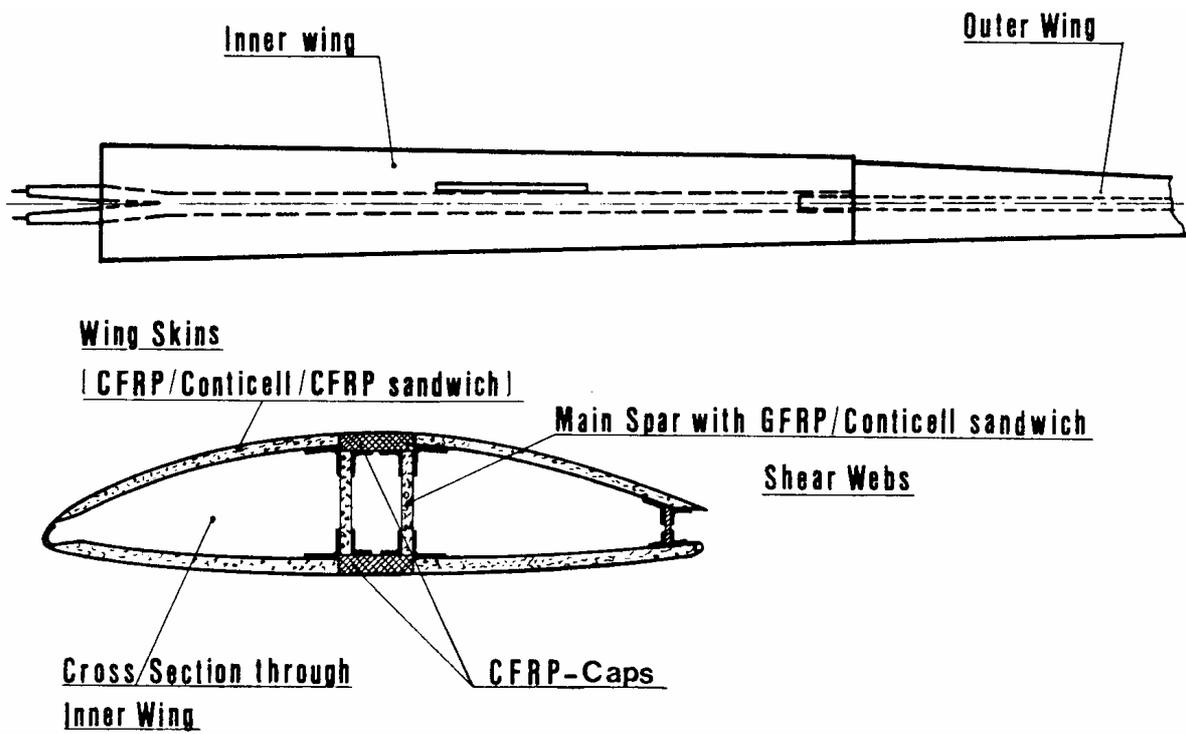
Figure 2: Structural details of a typical sailplane wing
