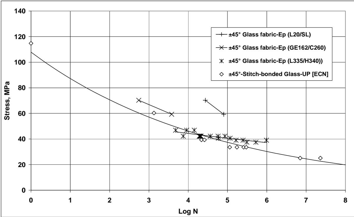
Figure 14: S-N curves for shear loaded  $\pm 45^\circ$  GFRP at  $R=-1$
