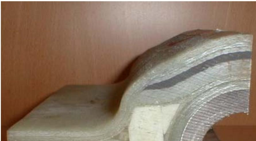
Figure 19: Picture of hybrid laminate in a stud joint [24]
