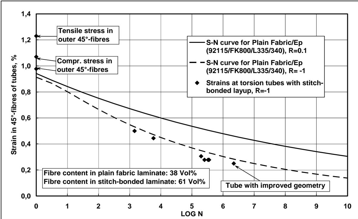
Figure 11: Fibre strain versus log N for torsion tubes with  $\pm 45^\circ$  lay-up
