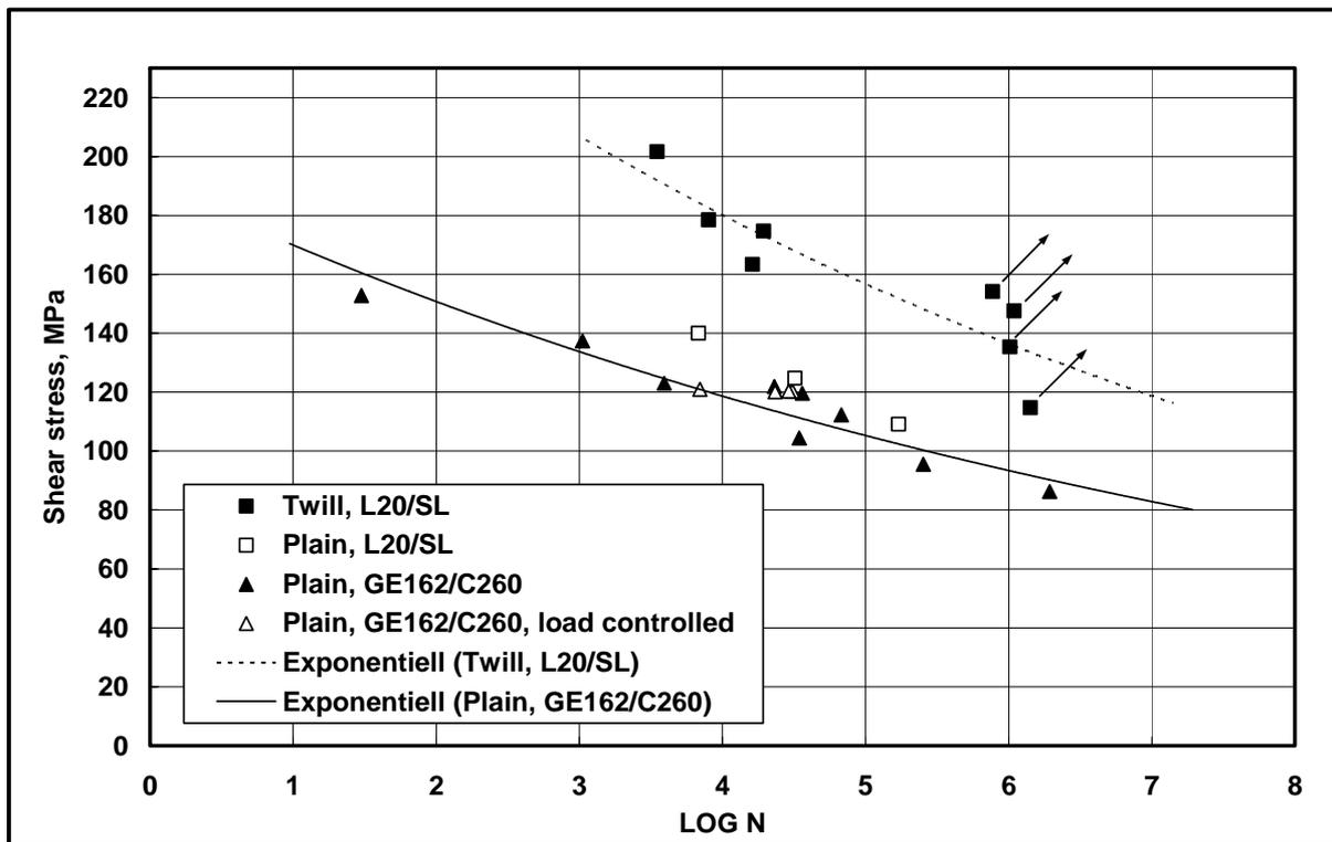
Figure 10: Fatigue behaviour of torsion loaded GI-Ep tubes with different undulation,  $R=0.1$  [14]
