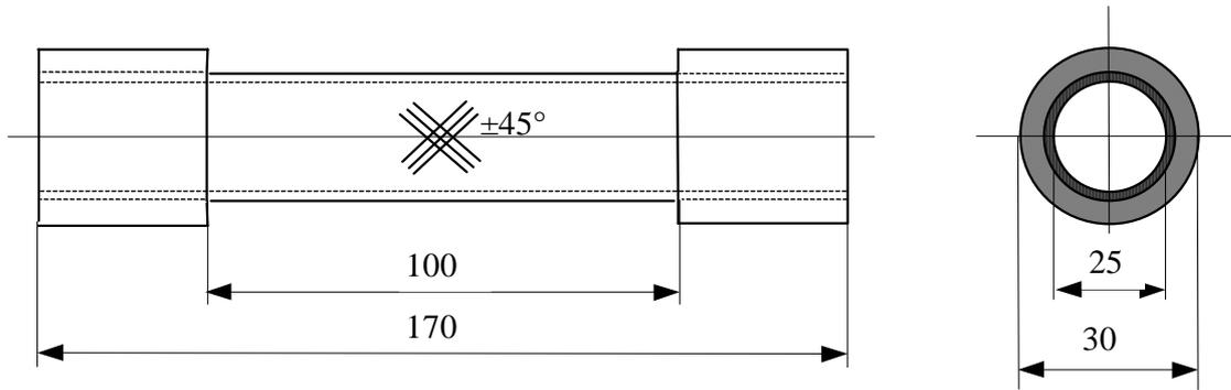
Figure 9: Geometry of  $\pm 45^\circ$  torsion tubes
