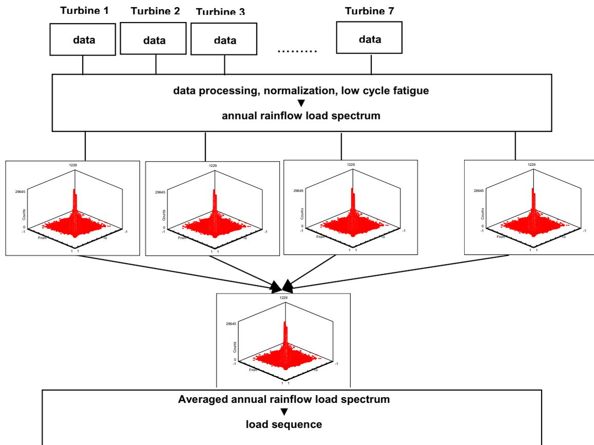
Fig. 1: Data Processing Scheme for NEW WISPER Synthesis
