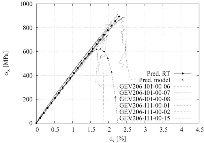
Figure 4: Predictions of strain-stress behavior of UD laminates in tensile test compared with experimental data, Pred. RT – predictions using experimentally measured  $\alpha_{11}^{(1)}(\varepsilon_1)$  for reference conditions, Pred. model- predictions using calculated (predicted)  $\alpha_{11}^{(1)}(\varepsilon_1)$ .
