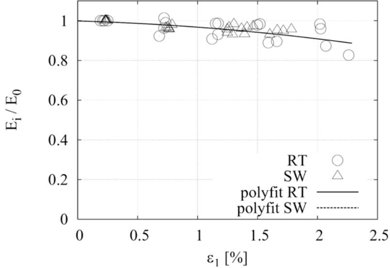
Figure 2: Stiffness degradation of UD composite. The second order polynomial,  $y = a_2x^2 + a_1x + a_0$  is used for approximation. The calculated constants are,  $a_0 = 1.0$ ,  $a_1 = -1.76$  and  $a_2 = -136.9$ .
