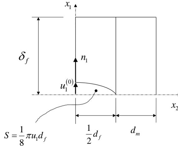
Figure 2. Representative volume element.  $\delta_f$  is ineffective length,  $d_f$  is diameter of the fiber,  $d_m$  is dimensions of the surrounding matrix, and  $S$  is  $1/4$  of the area of the ellipse under the crack profile line. The dimensions are calculated based on the fiber packing in hexagonal array.
