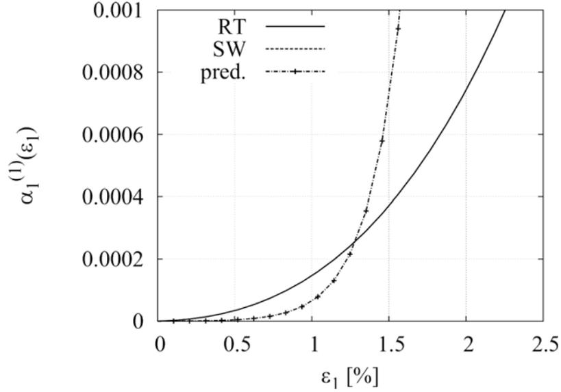
Figure 3: Calculated ISV  $\alpha_{11}^{(1)}(\varepsilon_1)$ , RT-reference material tested at ambient room conditions, SW-the same material that has been exposed to the salt water for 6month (tested at ambient room conditions).
