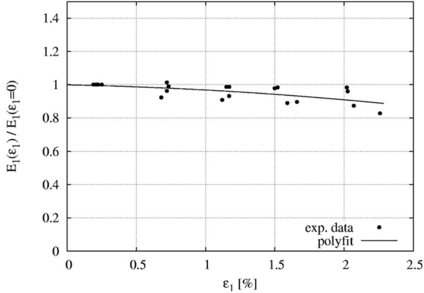
Figure 2: Stiffness degradation of UD composite. The second order polynomial,  $y = a_2x^2 + a_1x + a_0$  is used for approximation. The calculated constants are,  $a_0 = 1.0$  ,  $a_1 = -1.76$  and  $a_2 = -136.9$ .
