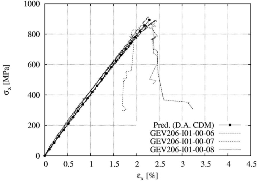
Figure 4: Predictions of strain-stress behavior of UD laminates in tensile test compared with experimental data.
