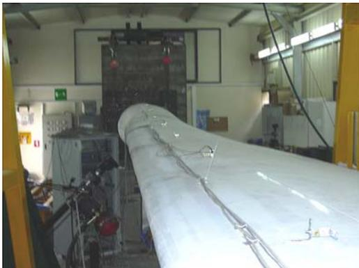
Figure X DAMPBLADE: Prototype damped blade tested
