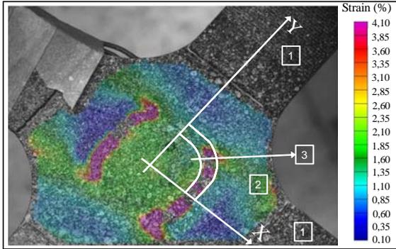
Figure X OPTIMAT BLADES: Comparison between isochromatic image and FE analysis of a bi-axially loaded cruciform specimen
