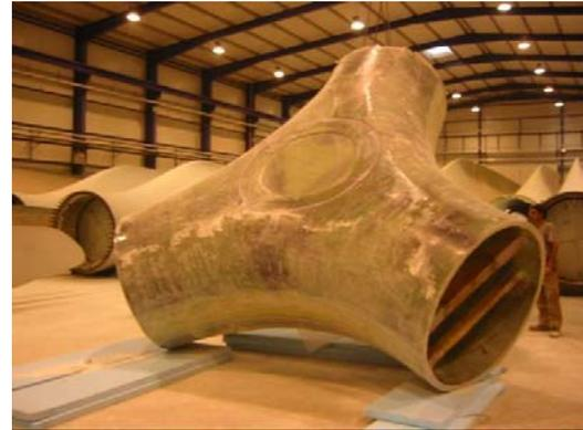
Figure X COMHUB: manufactured composite hub
