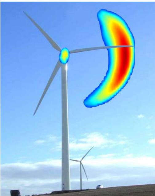
Figure X SIROCCO: Noise generated by wind turbine
