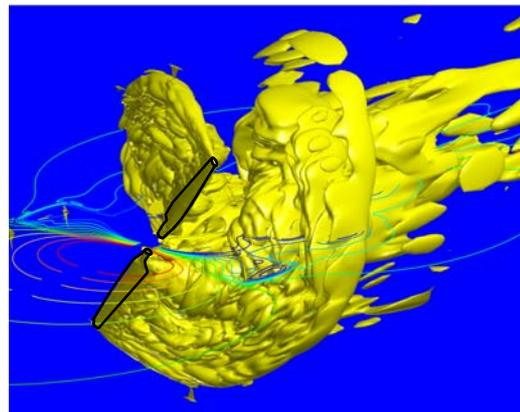
Figure X KNOW-BLADE: Vortex wake behind the NREL-Phase-VI rotor computed with the Detached Eddy Simulation technique
