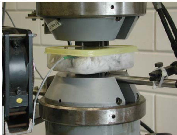
Figure 1 Test set-up for 100% relative humidity
