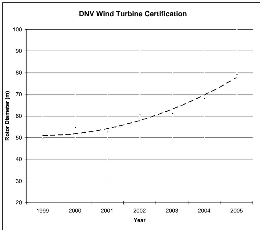
*Figure 1 - DNV Certificated turbines by diameter (excluding prototypes)*
