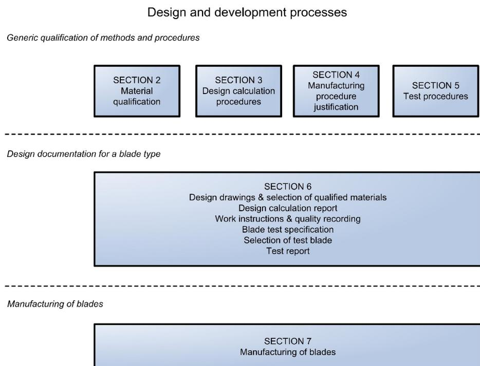
**Figure 2- Wind turbine design and development processes**
