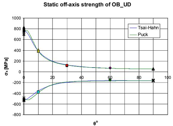
Figure 4 Static strength as a function of the angle between load and fibre direction
