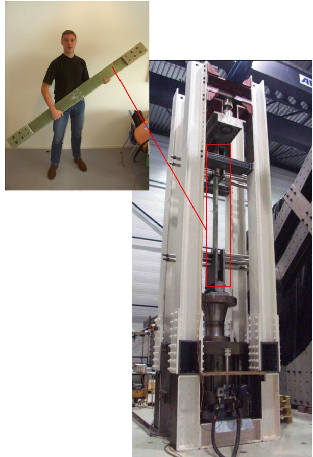
Figure 7 2500 kN test machine and test specimen
