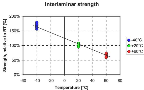
Figure 6 Interlaminar strength vs. Temperature
