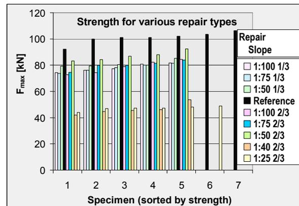
Figure 8 Influence of repair slope on static strength
