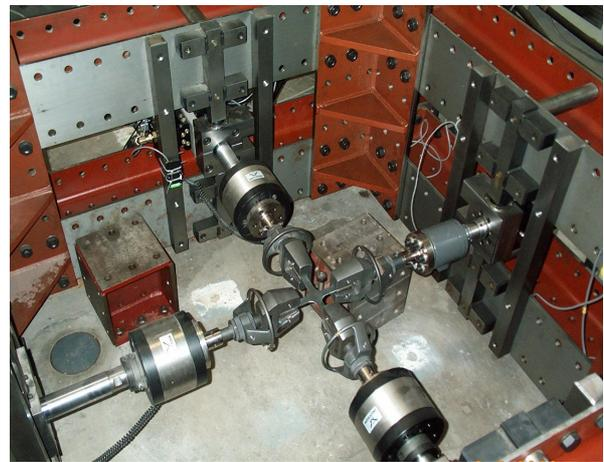
Figure 5 Bi-axial test set-up
