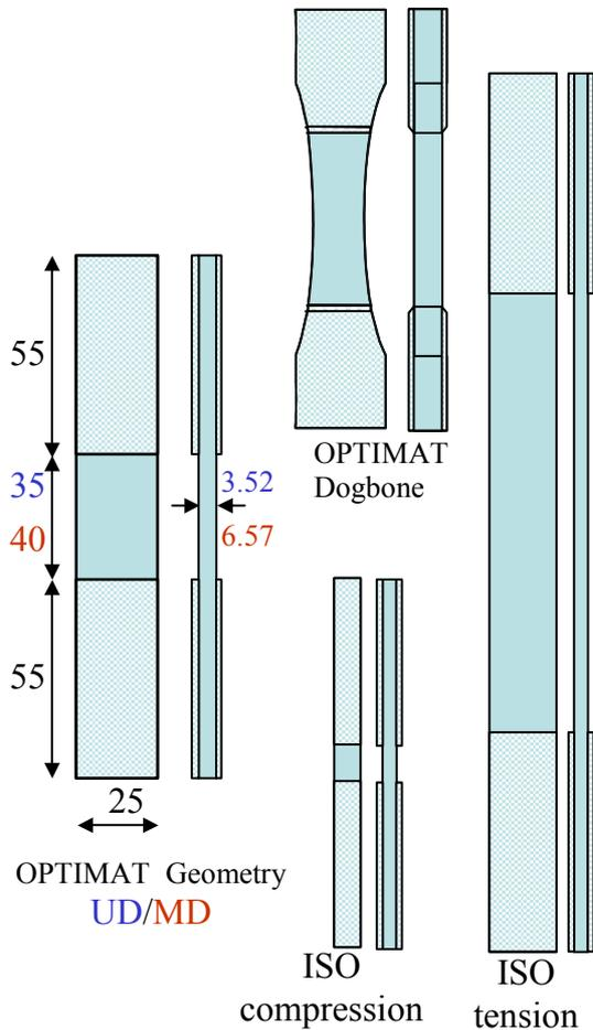
Figure 10 Some geometries used in the OPTIMAT BLADES project
