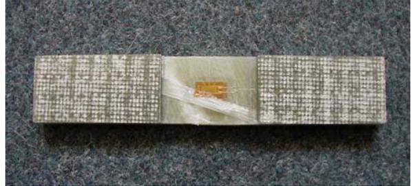
Figure 25: Failed MD coupon loaded off-axis in tension at 60°.
