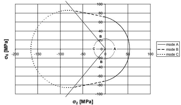
Figure 3: Failure locus in the ( $\sigma_2$ ,  $\sigma_6$ ) stress space, predicted with Puck failure criterion.
