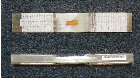
Figure 18: Failed MD coupon in tension. Furthermore, coupon catastrophic failure occurs in the tab area and this is correctly predicted by the FEM model, see Fig.17.
