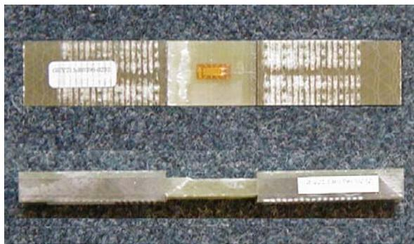
Figure 10: Front & Lateral side of a failed  $[90]_7$  coupon in compression.
