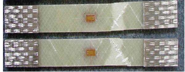
Figure 7: Upper & Lower faces of a failed  $[\pm 45]_s$  coupon, under tensile loading.
