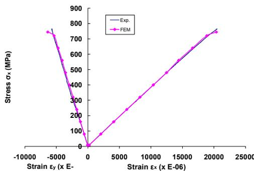
Figure 11: Stress-Strain behavior of a  $[0]_4$  coupon in tension.
