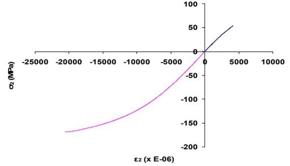
Figure 1: Tension-compression in the transverse to the fiber direction for UD Glass/Epoxy
