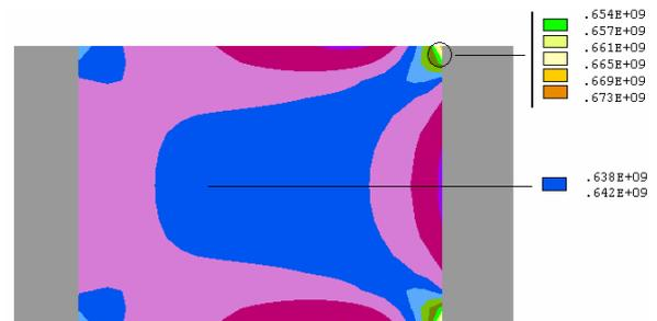
Figure 12: Normal axial stress distribution in the gauge area of a  $[0]_4$  coupon in tension.
