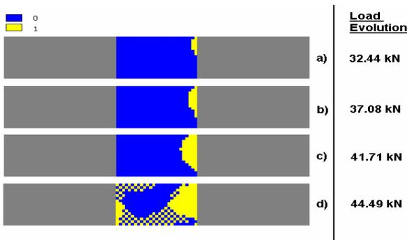
Figure 24: Damage evolution in the outer [15] ply of the MD 60 coupon.
