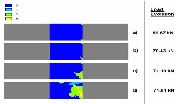
Figure 21: Damage evolution in the outer [55] layer of the MD coupon
