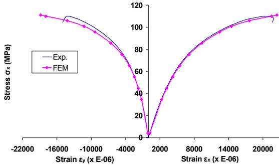
Figure 5: Stress-Strain behavior of a  $[\pm 45]_s$  coupon.
