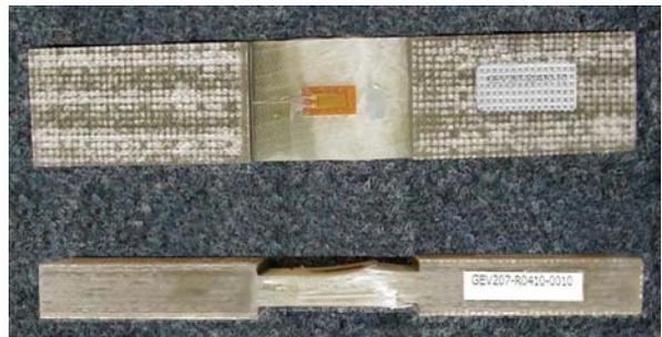
Figure 22: Failed MD coupon loaded off-axis in compression at 10°.
