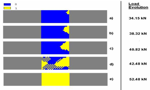
Figure 17: Damage evolution in the  $[45]$  layer of the MD coupon.
