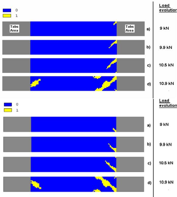
Figure 6: Predicted damage propagation in the 1<sup>st</sup> and 2<sup>nd</sup> layers of a  $[\pm 45]_s$  coupon under tensile loading.
