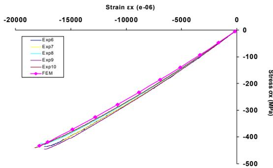
Figure 19: Stress-Strain behavior of an MD [10] coupon in compression.
