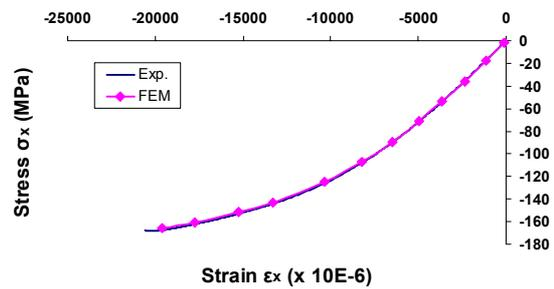
Figure 8: Stress-Strain behavior of a  $[90]_7$  coupon in compression.
