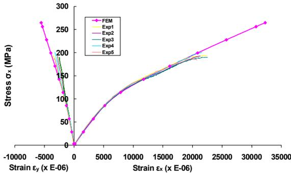
Figure 23: Stress-Strain behavior of an MD 60 coupon in tension.
