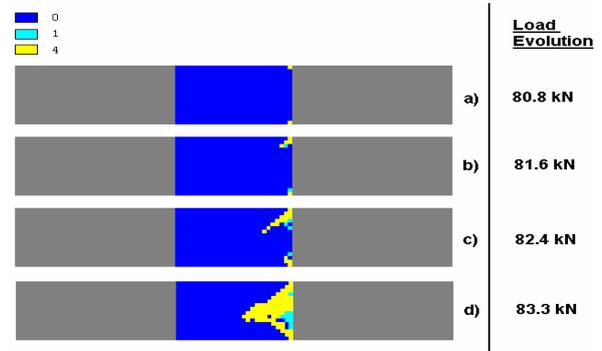
Figure 16: Damage evolution in the upper  $[0]$  ply of the MD coupon.
