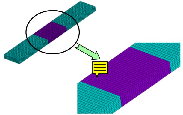
Figure 4: FEM model of a test coupon.
