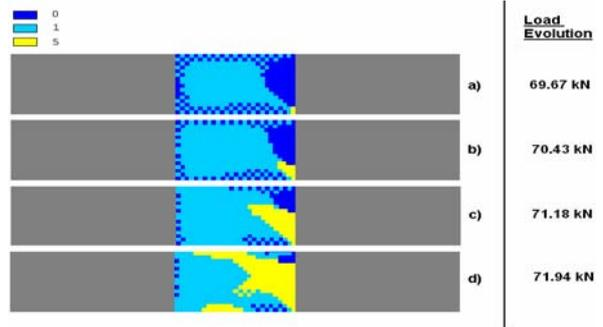
Figure 20: Damage evolution in the upper [10] layer of the MD coupon off-axis compressed.
