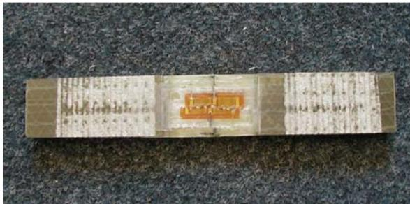
Figure 14: Failed  $[0]_4$  coupon in tension.
