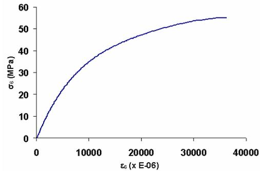
Figure 2: Shear stress-strain behaviour of UD material.
