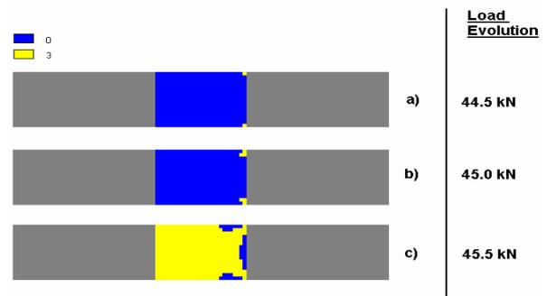
Figure 9: Predicted damage propagation in a  $[90]_7$  coupon under compressive loading.
