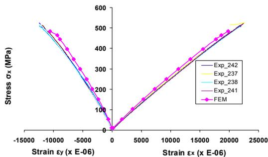
Figure 15: Stress-Strain behavior of an MD coupon in tension.
