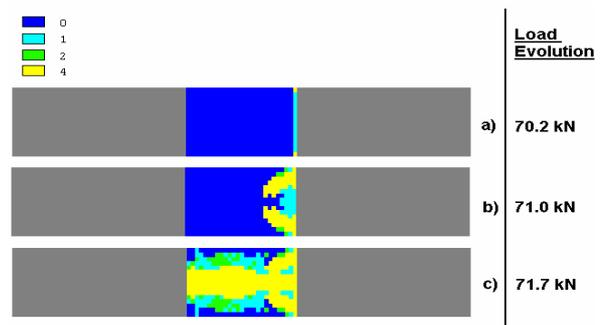
Figure 13: Predicted damage propagation in the UD  $[0]_4$  coupon.
